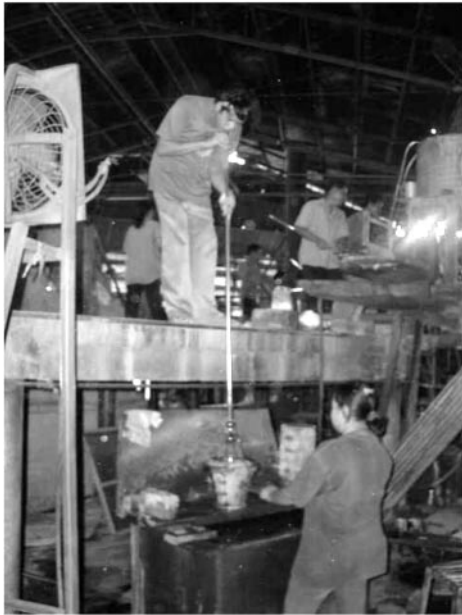
Fig. 3. Blowing melted glass to shape a lump bulb. On the stage a worker blow the air into the melted glass to shape a bulb. On the flow another worker holds a mold.
