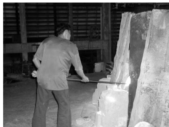
Fig. 2. Work to take out glass from the furnace to make a bulb.
