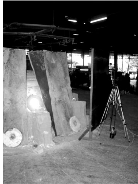
Fig. 4. Measurement of thermal condition behind a heat barrier.
